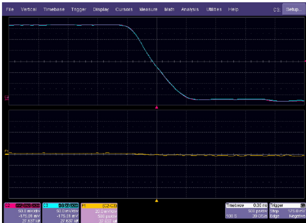
Figure 11. Channels after skew adjustment, F1 trace appears flat after adjustment
